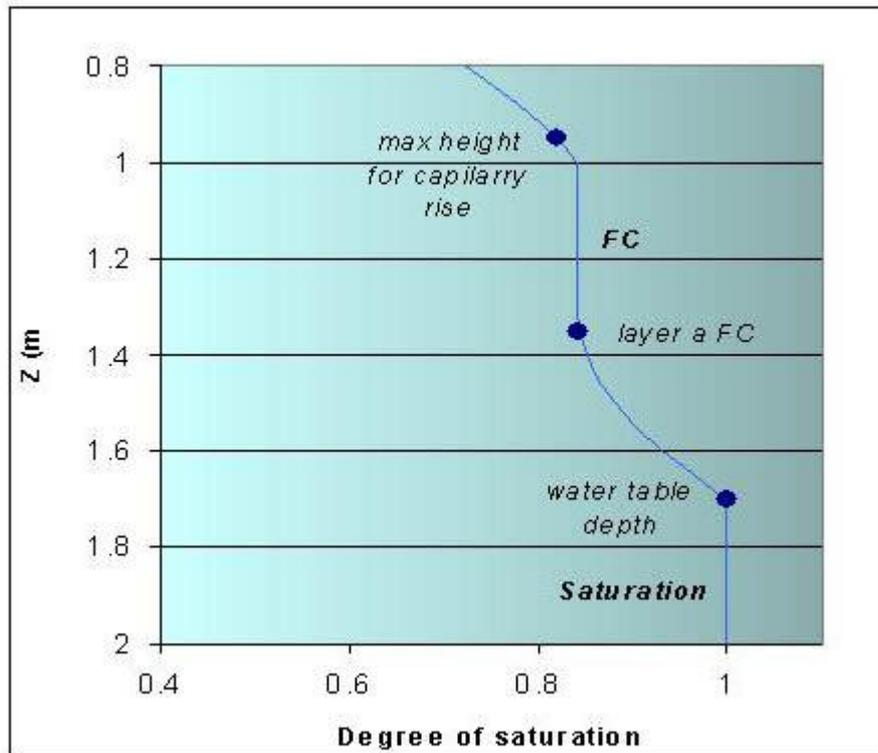
Figure 0-7. Trend of the relative humidity of the soil values ( $\theta/\theta_s$ ) in the presence of water. The capillary rise takes effect from the deepest layer to field capacity: profile of soil affected by the rise is brought to FC.
