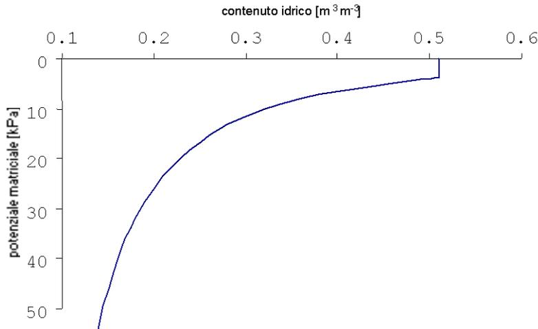
Figure 2-2. Example Campbell soil water retention curve near saturation.
