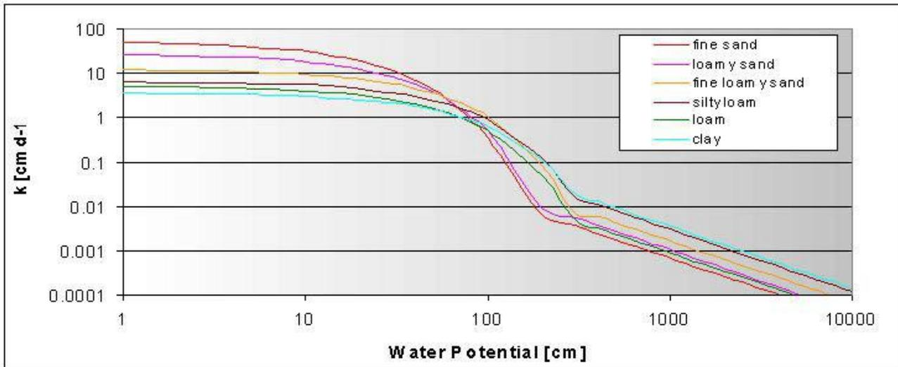
Figure 0-10. hydraulic conductivity ( $K$ ,  $\text{cm d}^{-1}$ ) for soils with uniform texture.
