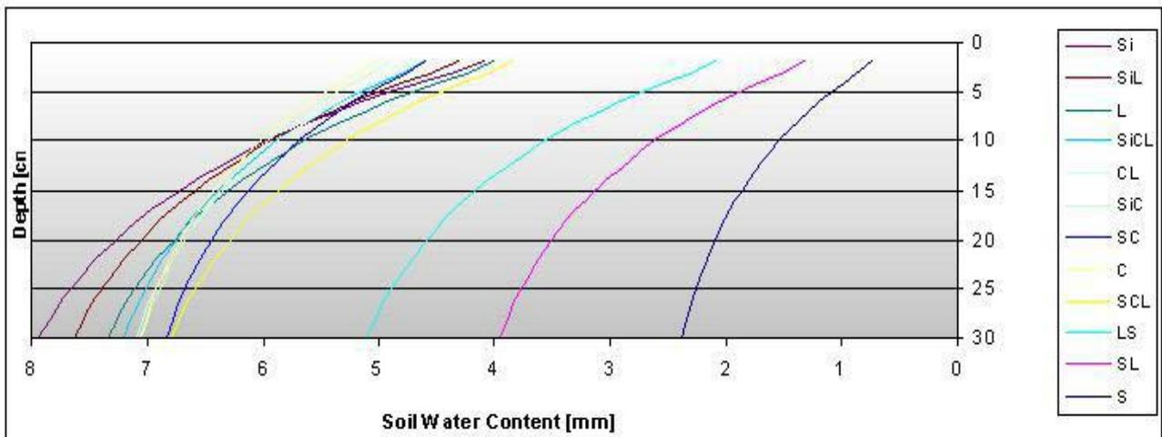
Figure 0-15. Threshold of evaporation in the first 30 cm of the profile for all textual classes. ( S=sandy, SL=Sandy Loam, LS=Loamy Sand, SIL= Silty Loam, L=Loam, Si=Silty, SCL=Sandy Clay Loam, SiCL=Silty Clay Loam, CL=Clay Loam, SC= Sandy Clay, SiC= Silty Clay, C=Clay).
