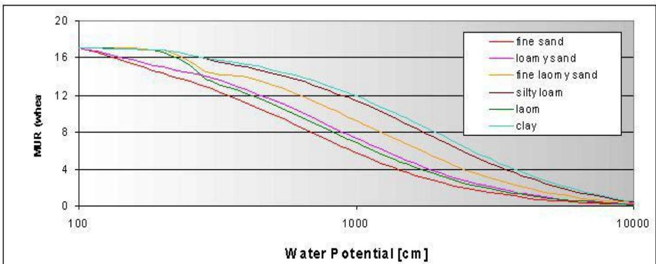
Figure 0-12. Levels of MUR (maximum uptake rate) in for a uniform soil profile of 1 m, under wheat crop.
