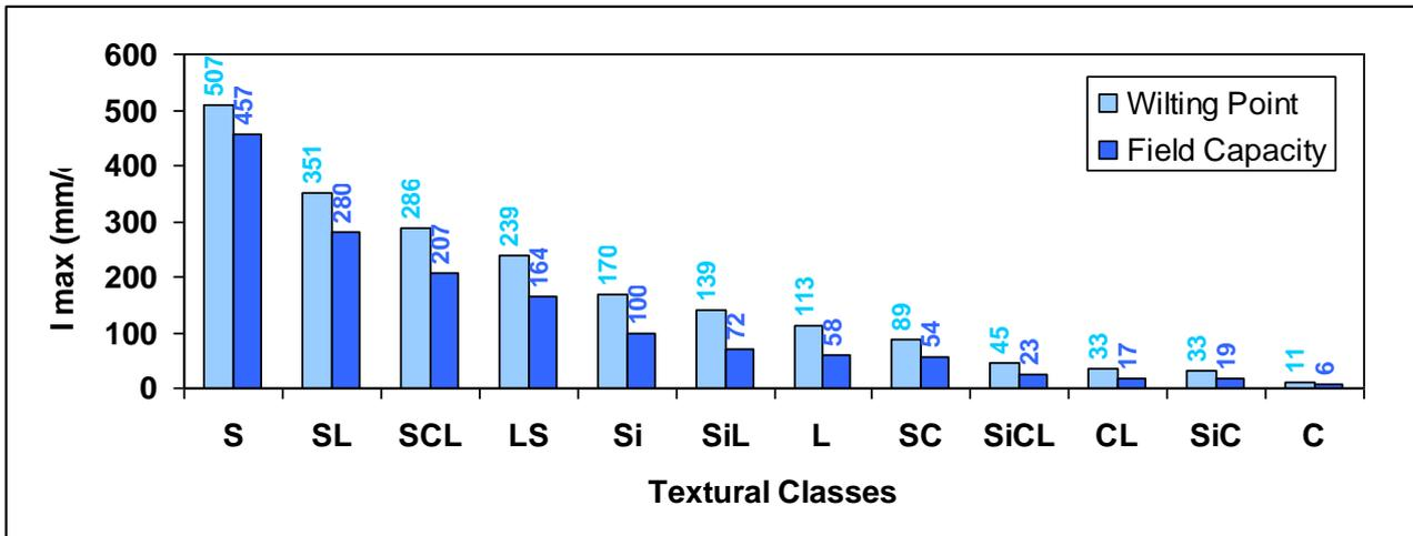
Figure 0-2. Maximum infiltration ( $I_{max}$ ) after a day of rain at field capacity (FC) and wilting point (WP) for the different textures (S=sandy, SL=Sandy Loam, LS=Loamy Sand, SiL= Silty Loam, L=Loam, Si=Silty, SCL=Sandy Clay Loam, SiCL=Silty Clay Loam, CL=Clay Loam, SC= Sandy Clay, SiC= Silty Clay, C=Clay).
