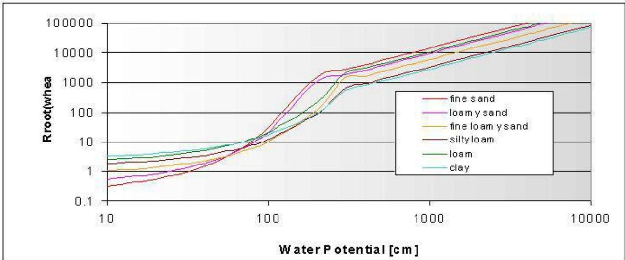
Figure 0-11. Values of the variable *Rroot* as a function of the potential in uniform soils cultivated with wheat.
