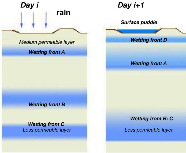
Figure 0-4. infiltration into the soil profile of moisture fronts A,B,C,D.
