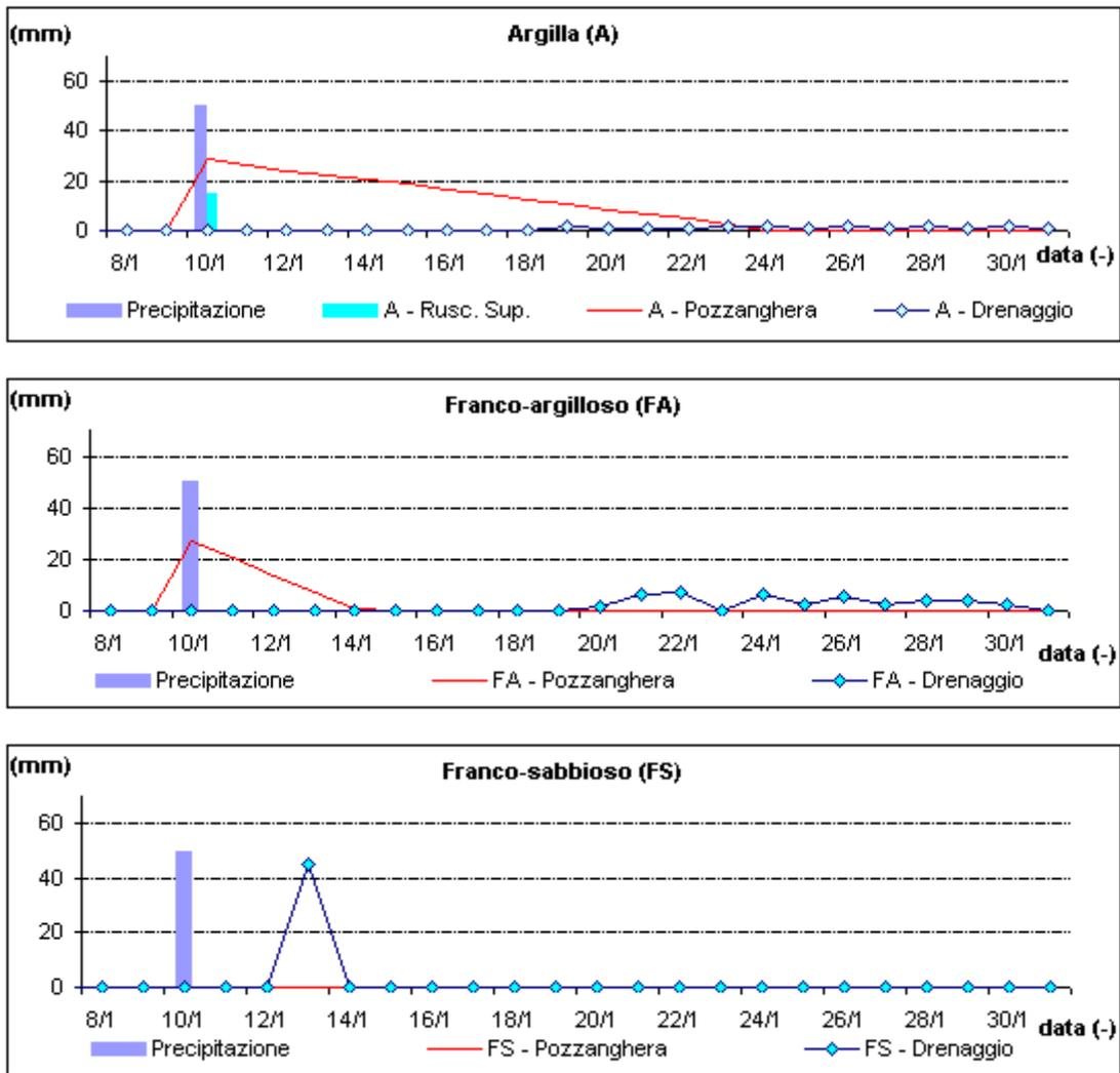
Figure 0-5. Time trends in the pond, surface runoff and deep drainage after a rain event of 50 mm (10 January) for three types of soil (C clay, CL loamy-clay, LS loamy-sand).
