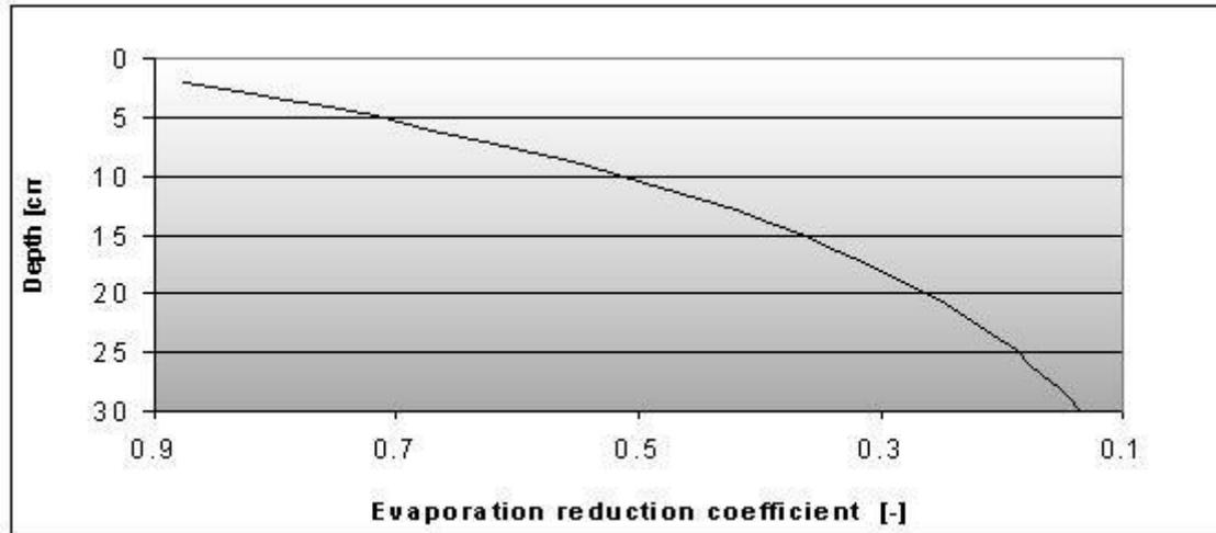
Figure 0-16. Reduction of evaporation in the first 30 cm of the profile for all textual classes.
