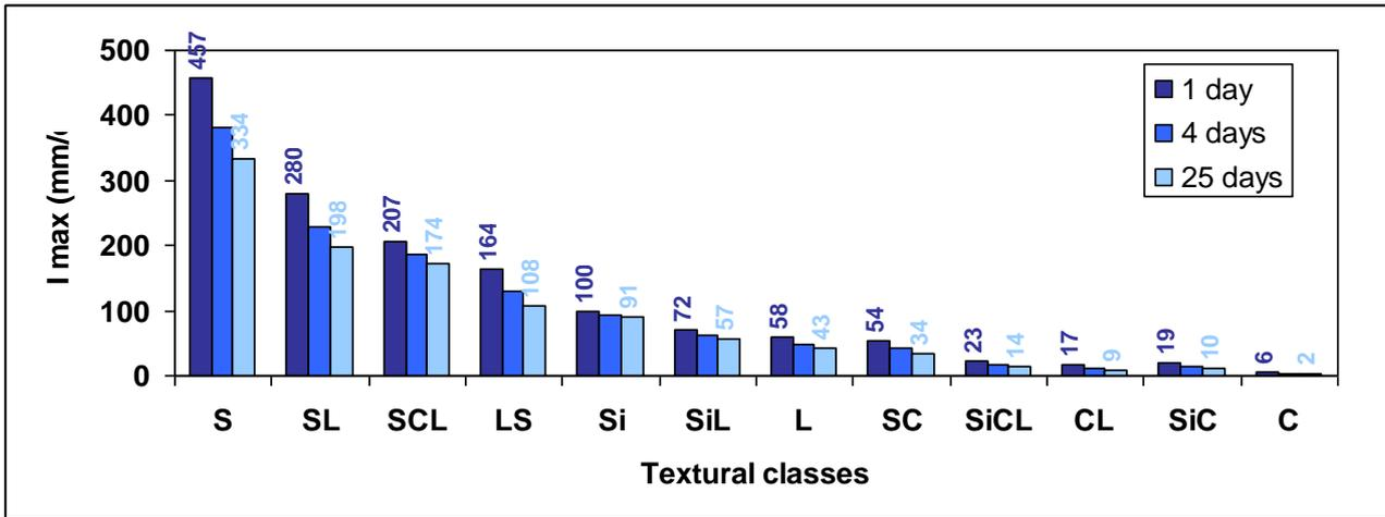
Figure 0-3. Maximum infiltration ( $I_{max}$ ) consequently to the number of days since last rain (Water content = field capacity).
