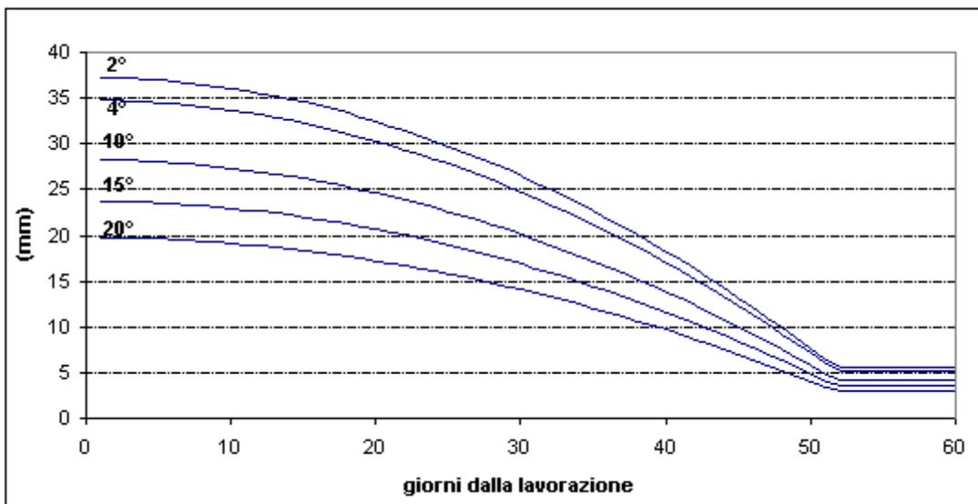
Figura 0-6. Height of storage surface: effect of the surface slope.
