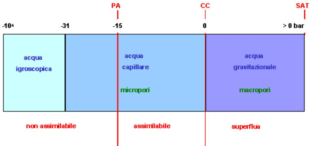
Figure 2-1. Characteristic levels of the water retention curve with their types and levels of water availability for crop
